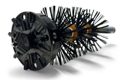
Featuring our Driller Head in the front and a Cutting Plate with our carbide star tips, this Cutter is designed to remove collapsed liner and concrete. It can also be used as a lateral cutter and the best part is that the Driller Head and the plate is easily replaceable.
