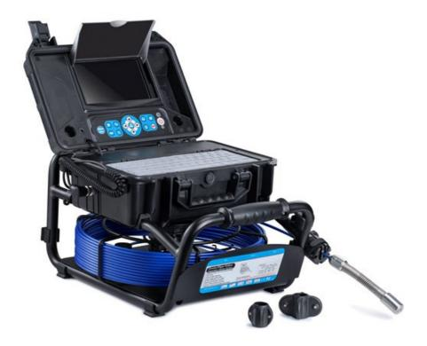
The 3499F camera is an affordable, lightweight push-rod camera system for inspection sewer lines from diameters 40 mm to 150 mm. Equipped with a 23 mm camera head that is waterproof to depths of 10 m, with a 120° wide-angle lens, 12 LED lights and sapphire glass cover, makes it the perfect addition to any drainage vehicle. The perfect camera to use to see before/during/after cleaning work with our high-speed machines.
